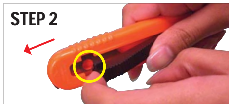
Push forward the black slider until aligned with rectangular slot.
