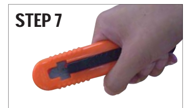
Push the black slider back into the rectangular slot.
