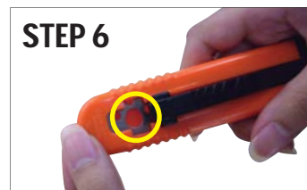
Load blade until centre hole aligns with rectangular slot.
