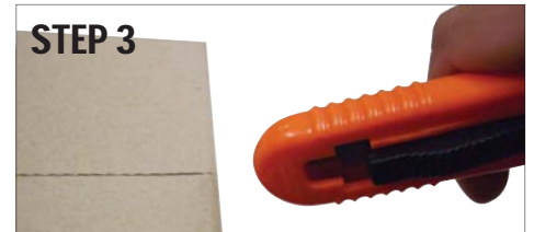
Blade automatically retracts after cutting. This prevents accidents.
