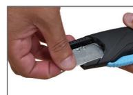
4. Carefully place the blade into position
