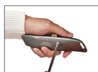
1. Use a Phillips screwdriver to unscrew.
