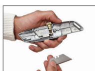
3. Insert a new blade
